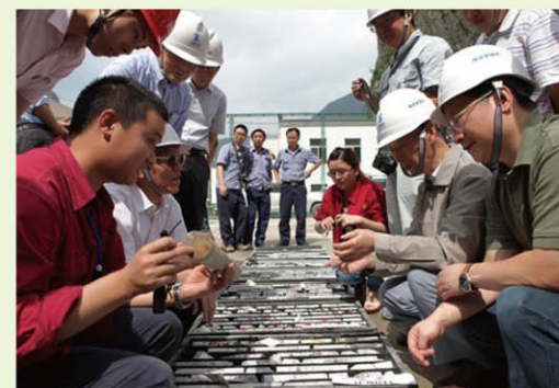
查勘锦屏一级水电站大坝芯样
